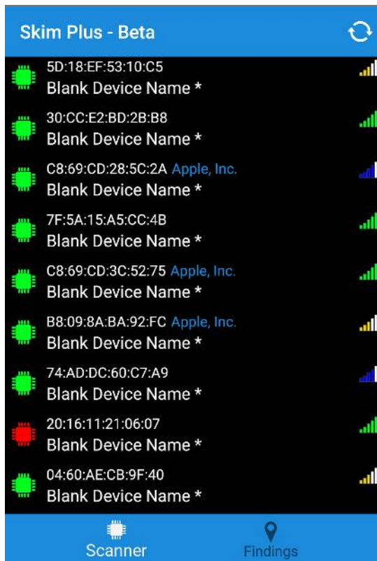
Fig. 5: This is a screenshot of a Google Pixel 2 running App C while Skimmer S-02 is powered on. The skimmer is the device second from the bottom of the list. The app indicates that the device is a skimmer by assigning it a red icon instead of green. This app also listed 14 other devices in this running instance that are not shown in this image; the user must scroll through the list to find the detected device.
