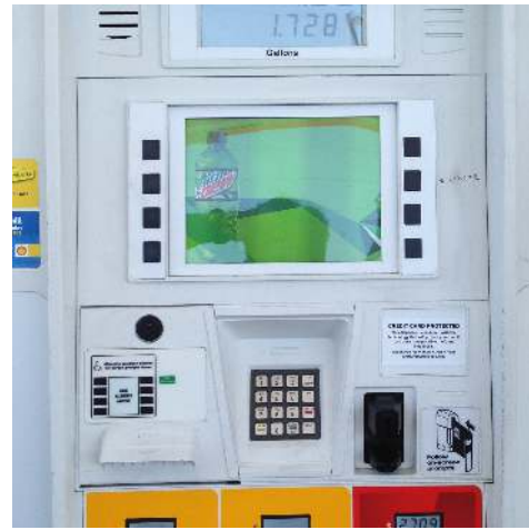
(b) This pump has no seal.
